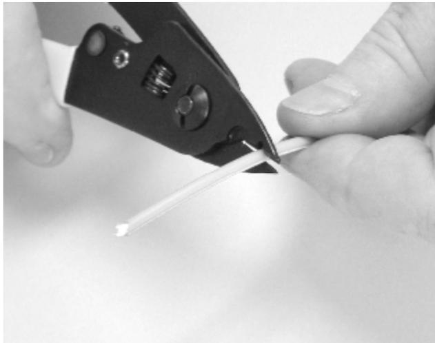
Place the cable in the large notch and close the stripper firmly to sever the cable jacket. Grasp the jacket with two fingers, rotate to make sure it is severed completely and pull off gently.
