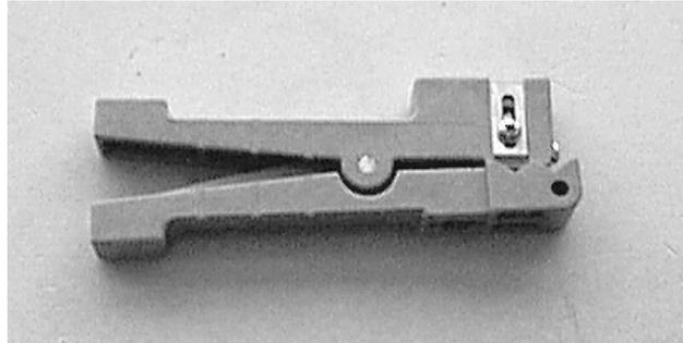
This lightweight stripper will make round or axial cuts on jacket/buffer tubes quickly and easily. The adjustable blades can be set to any depth from 1/8in. to 7/32in. (3.175mm to 5.556mm) to assure nick-free strips. Each stripper comes complete with one round and three straight blades.
