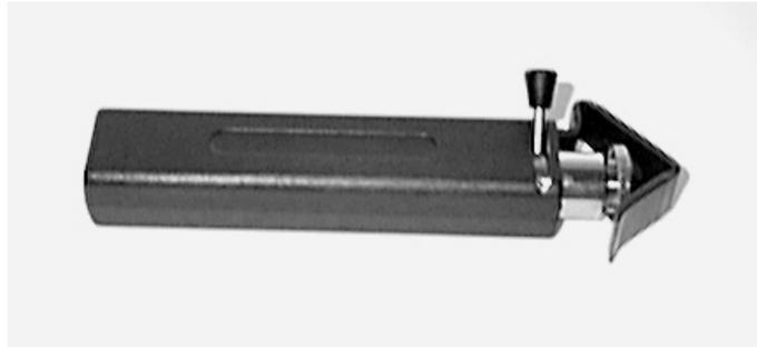
The Cable Slitting and Ringing tool can be used on cable with an outside diameter of up to 2.75in. The blade is adjustable for jacket thickness' up to 0.187in.. The blade can be turned 90 degrees for an axial cut, left in its normal position set for a round cut or changed to a 'in between' angle for a spiral cut. A spare blade is stored in the handle.
