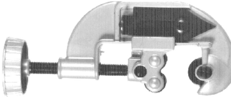
This tubing cutter can be used with 1/8" to 1 1/8" outside diameter armored cables. It features an alloy steel cutting wheel and two grooved rollers for cutting through both outside jacket and armor.
