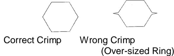
If the finished crimp looks like the one pictured above right, an over sized crimp ring was used. Completing the crimp will damage the tool. Check with the connector manufacturer for the proper crimp ring size.
