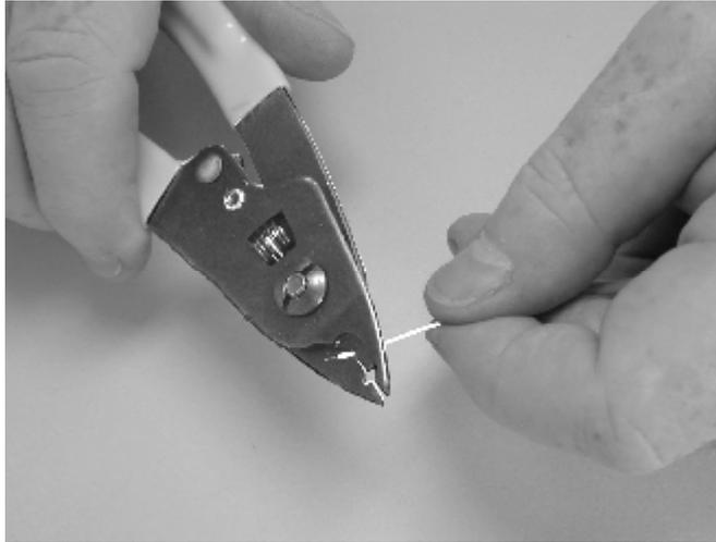
Rather than stripping the fiber completely at one time, which may break the fiber, strip in several short strips of about 1/8" (3 mm) at each time until you reach the desired finished length. This will relieve any pressure caused by the buffer as it bunches up ahead of the stripping tool.
