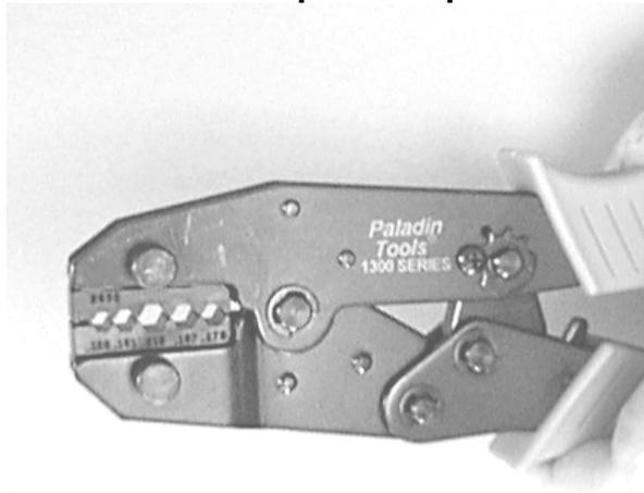
The crimp tool provides the proper compression force required to insure retention of the connector on the cable. The toggle action provides a very high mechanical advantage assuring a proper crimp each time. The ratchet feature means that once a crimping cycle is started, it must be completed, insuring a complete crimp.
