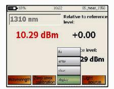
F4 "Light Source" enables the user to turn the 1310nm or the 1550nm light source on or off. Both wavelengths have two transmitting options either CW(constant wave) or 2Khz mode.
