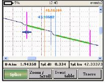
the event and the fifth marker (c) is used to locate the begining of the event. The measurement results are displayed in the horizontal information panel. The **SpI**, **dB** field in the information panel displays the attenuation of the event while the **SpI**, **km** field displays the distance to the event being tested (middle marker).
