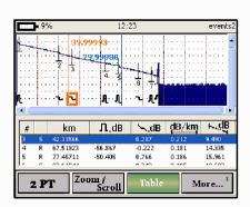
**Note:** User can still continue working with the trace while in the Event Table mode. F keys enabled functions include moving markers, zooming and scrolling.
