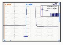
displays the attenuation between the left and right hand markers, while the **dB/km** field displays the attenuation coefficient.
