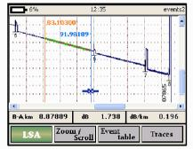
upon where the left hand marker (A) and right hand marker (B) are positioned on the trace screen. The dB field in the information panel displays the attenuation between the left (A) and right (B) hand markers, while the dB/km field displays the attenuation coefficient.
